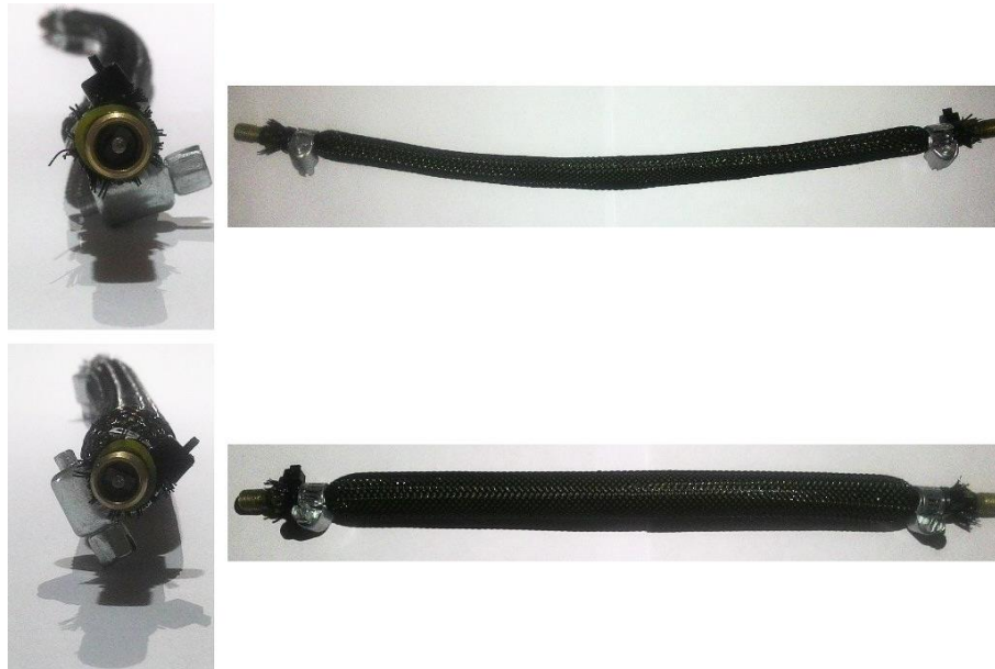
Figure 2. Comparison between air muscle depressurized (above) and pressurized (below).
