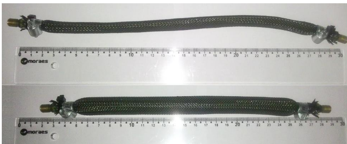
Figure 3: Measure of shift in air muscle depressurized and pressured.
