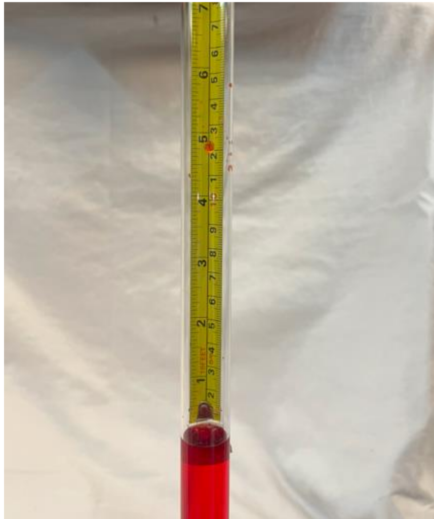
Figure 19. Acrylic tube with a scale behind it, connected to the bidet suction pump.
