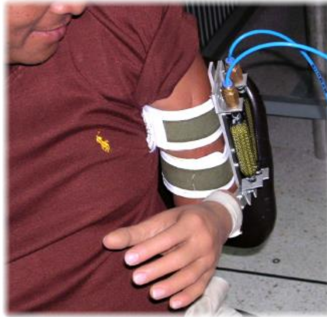
Figure 6. Prosthesis with McKibben actuators. Source: Laksanachaeoren & Wongsiri (17).
