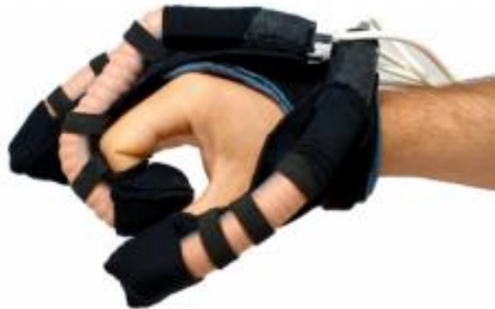
Figure 3. Electromagnetic pulses power the soft robot glove prototype. Source: Harvard Biodesign Lab (15).
