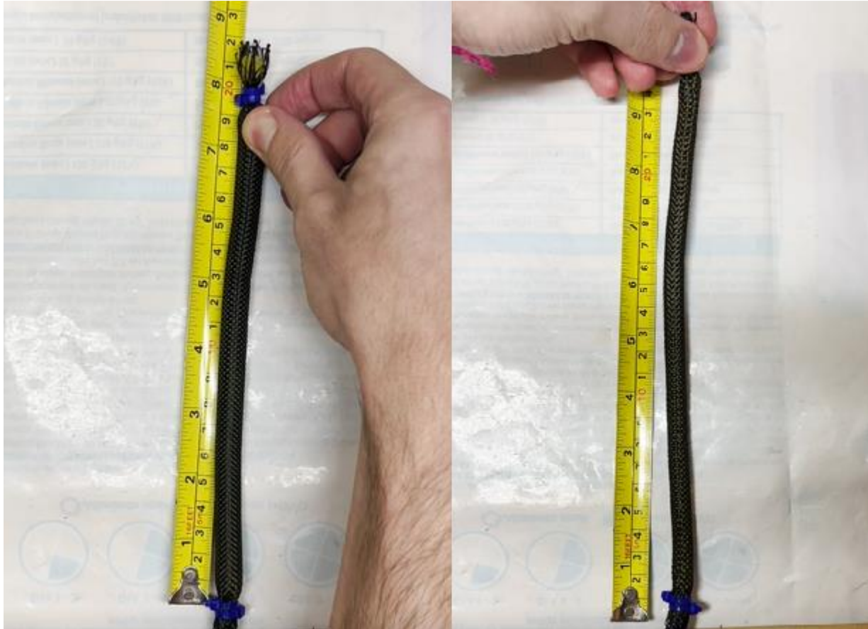
Figure 11. Demonstration of McKibben muscle activation. On the left, the actuator was activated under a 1.5 bar pressure.
