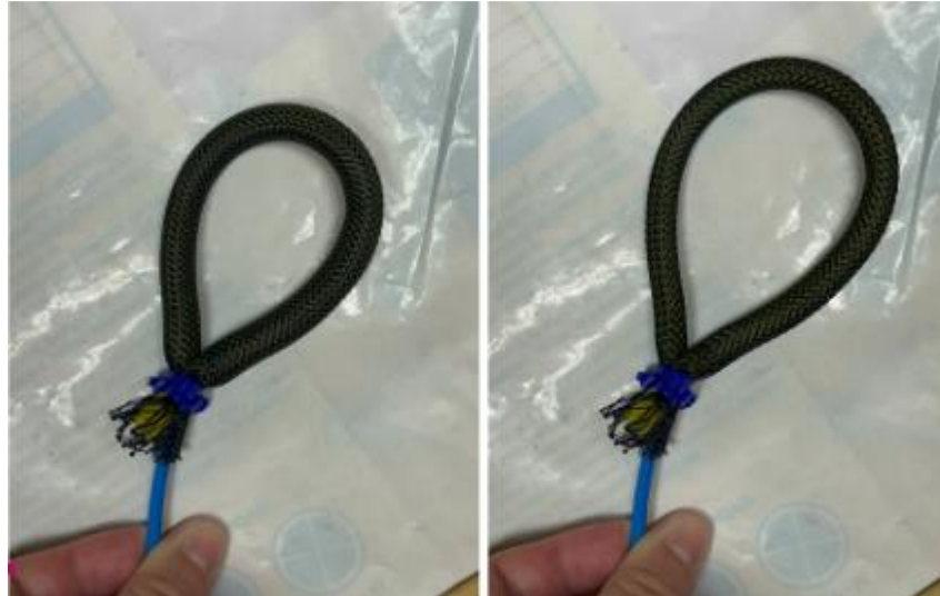
Figure 12. Demonstration of the activation of the circumferential McKibben muscle. On the left, the actuator was activated under a 1.5 bar pressure.
