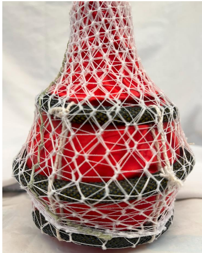
Figure 16. Circumferential arrangement of actuators in the compression movement demonstration.
