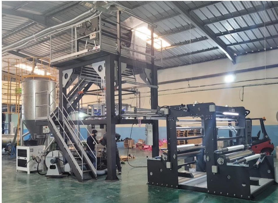
Figure 03. Photo of an industrial plant, containing a PVC film extrusion machine.
