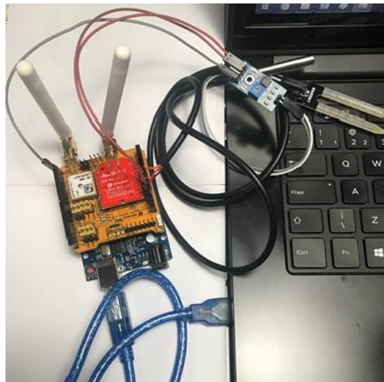
Figure 3. Photograph of the soil temperature and humidity sensors installed on the Arduino connected to the computer via USB cable.
