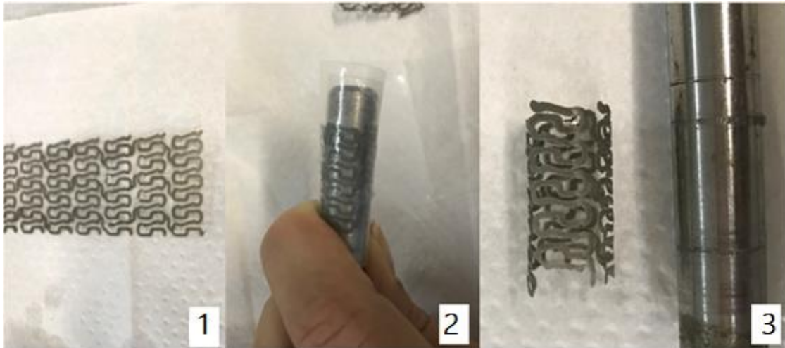
Figure 2: Item 1: Prototype after 3D printing, flat. 2: Prototype attached to the metallic guide. 3: Prototype after thermal shock, already in the shape of a tube.
